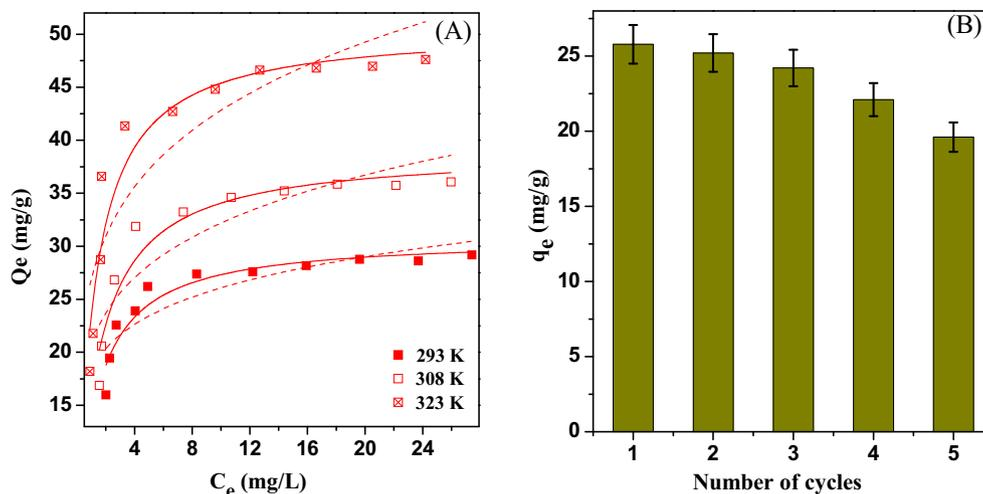
**Fig. 4.** (A) Sorption isotherms of U(VI) on MSD at three different temperatures, solid and dashed lines: Langmuir and Freundlich model, respectively. (B) Recycling of MSD for U(VI) removal using 0.5 mol/L  $\text{Na}_2\text{CO}_3$  as a desorption agent, pH = 5.0, m/V = 0.5 g/L,  $I = 0.01$  mol/L  $\text{NaNO}_3$  and  $T = 293$  K.
