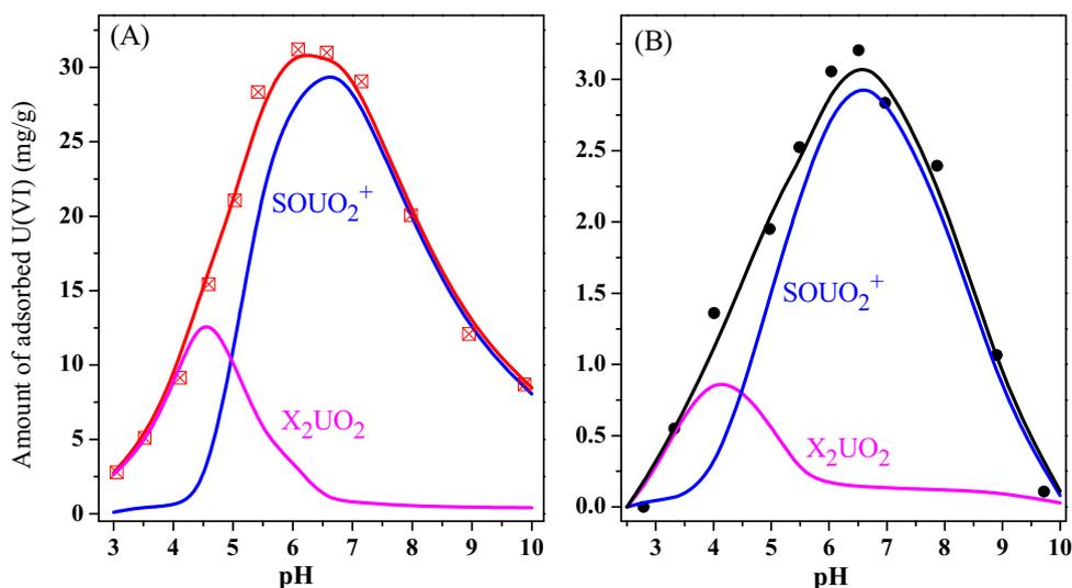
Fig. 6. Surface complexation modeling of U(VI) sorption on diatomite and MSD,  $C_0 = 24 \text{ mg/L}$ ,  $m/V = 0.5 \text{ g/L}$ ,  $I = 0.01 \text{ mol/L NaNO}_3$  and  $T = 293 \text{ K}$ .
