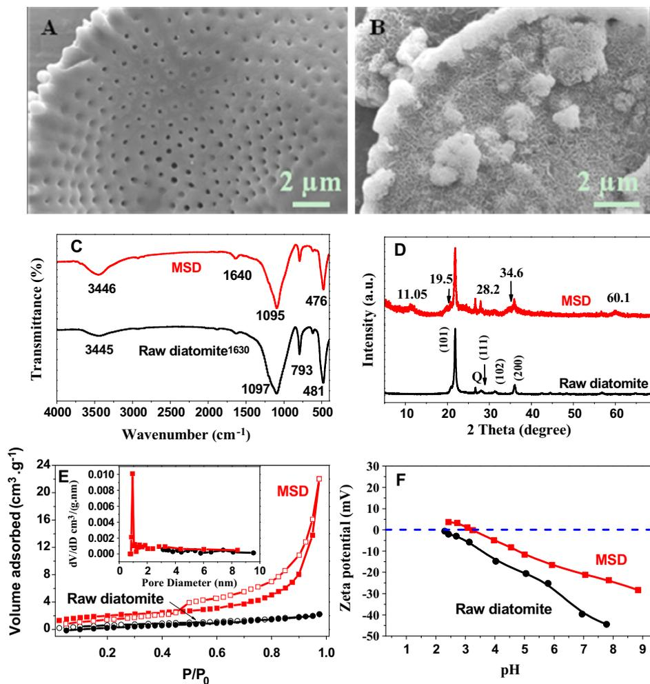
**Fig. 1.** Characterization of diatomite and MSD. (A and B) SEM images of raw diatomite and MSD, respectively; (C) FT-IR spectra; (D) XRD patterns; (E)  $N_2$  adsorption-desorption isotherms, the inserted curves: the distribution of pore size; (F) zeta potentials,  $m/V = 0.5$  g/L,  $I = 0.01$  mol/L  $NaNO_3$  and  $T = 293$  K.
