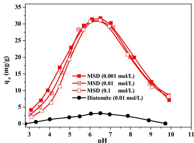
Fig. 3. Effect of pH on the sorption of U(VI) on diatomite and MSD.  $C_0 = 24$  mg/L,  $m/V = 0.5$  g/L and  $T = 293$  K.
