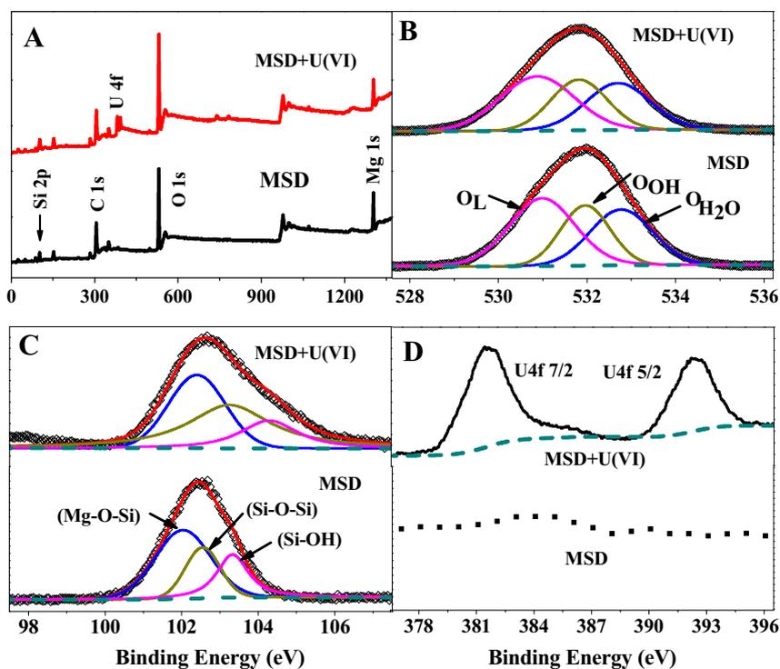
Fig. 5. XPS analysis of MSD before and after U(VI) sorption, (A) total survey; (B and D) high resolutions of O 1s, Si 2p and U 4f, respectively.
