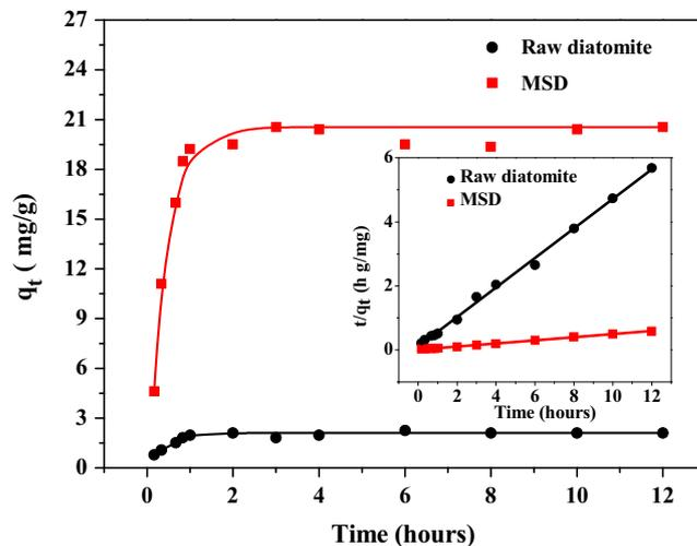
**Fig. 2.** Sorption kinetics of U(VI) on diatomite and MSD, inserted curve: the fitting of the pseudo-second order kinetic model,  $pH = 5.0$ ,  $C_0 = 24$  mg/L,  $m/V = 0.5$  g/L,  $I = 0.01$  mol/L  $NaNO_3$ ,  $T = 293$  K.
