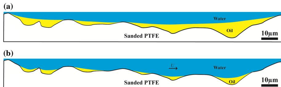
**Fig. 4** Lubricant pools on the PTFE surface sanded with grit designation of 240 grits (RMS roughness of 13.7  $\mu\text{m}$ ). This 150- $\mu\text{m}$ -long slice of the surface was taken from actual profilometry measurements. It is a representational slice of the sanded PTFE surface. Superimposed on the surface topography is a schematic diagram
